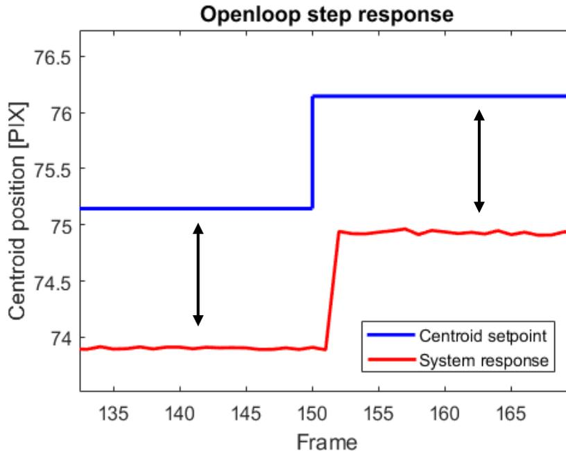
**Figure 33.** Step response in open loop
