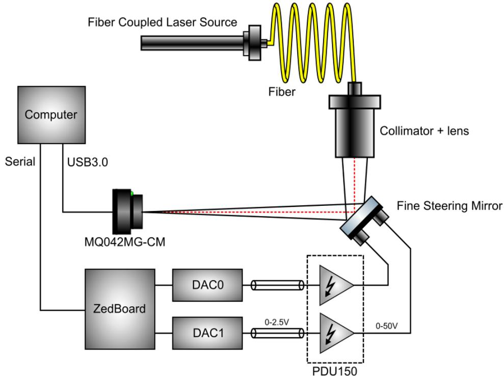
**Figure 13.** Graphical representation of the active correction setup
