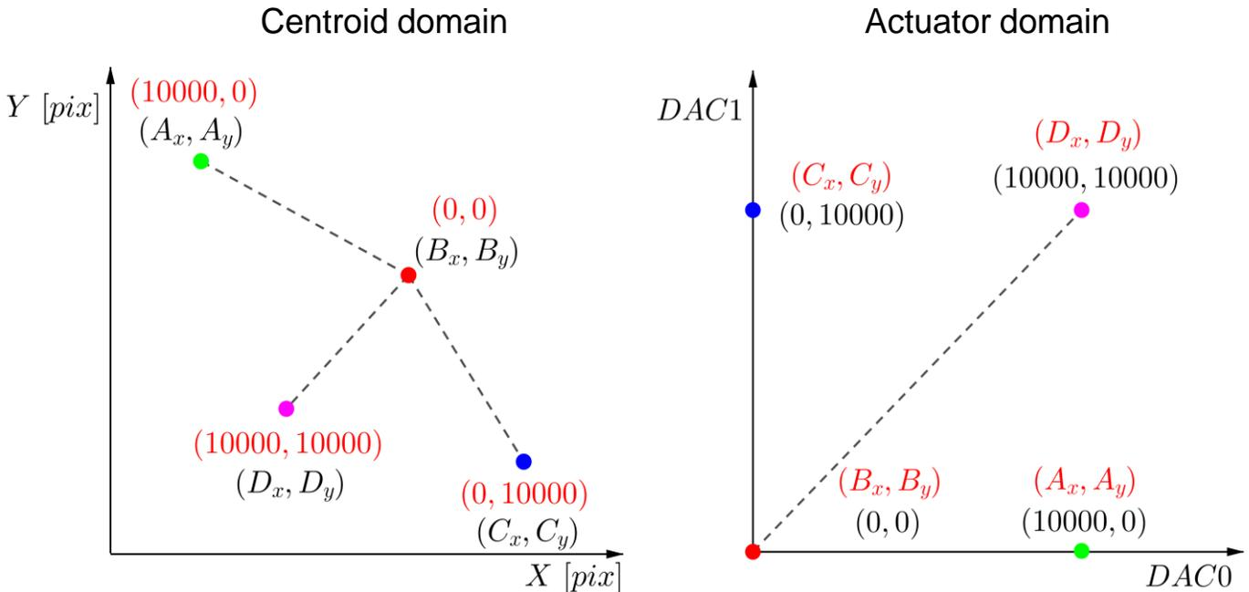
**Figure 22.** Affine transformation from warped centroid domain to actuator values
