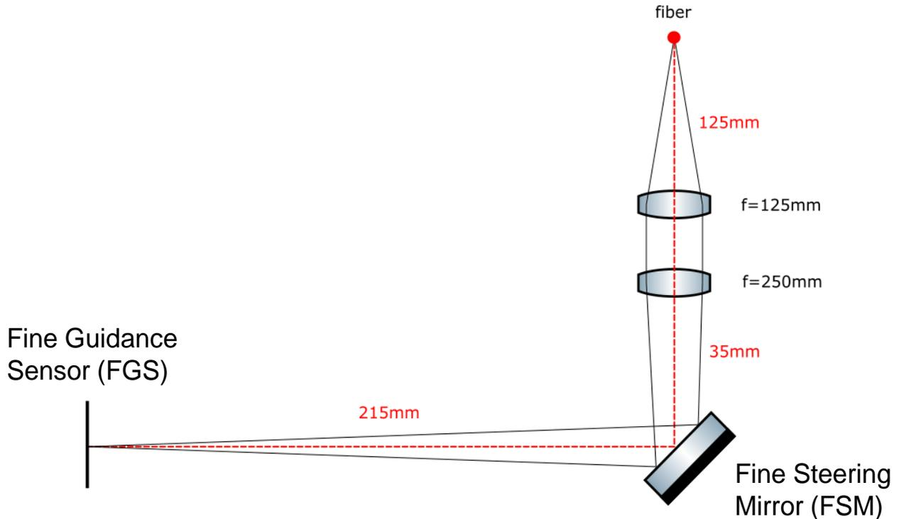
**Figure 14.** Optical configuration of the active correction setup
