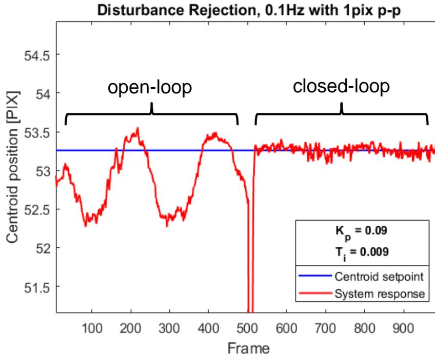
**Figure 36.** 0,1 Hz disturbance, ~1 pixel p-p magnitude, without and with closed loop enabled (framerate = 30 fps)
