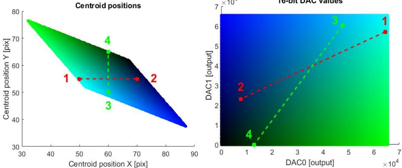
**Figure 27.** Horizontal and vertical centroid movement (left) linearly transformed to the cartesian actuator grid (right)
