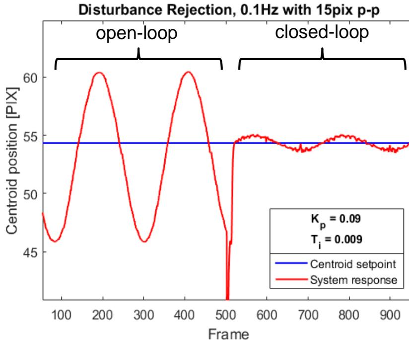
**Figure 37.** 0,1Hz disturbance with, 15 pixel p-p magnitude, without and with closed loop enabled (20dB attenuation)
