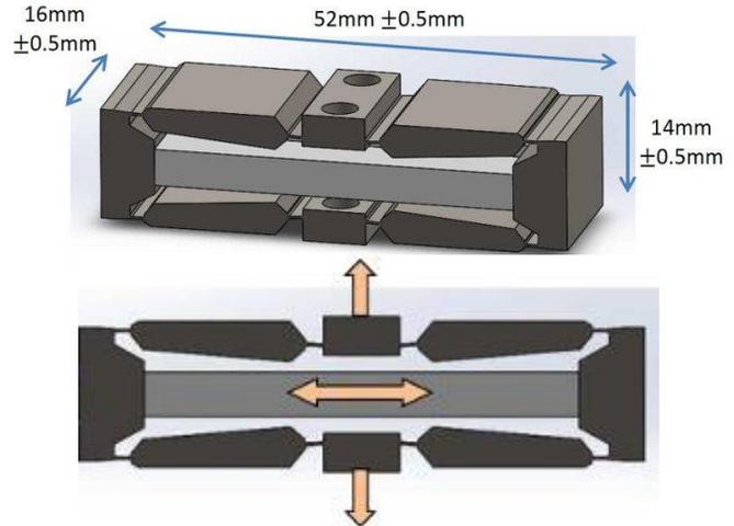
**Figure 20.** Amplified stack piezo actuator
