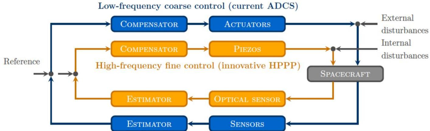
**Figure 11.** Control loop scheme with the active correction loop indicated in orange, ADCS loop in blue
