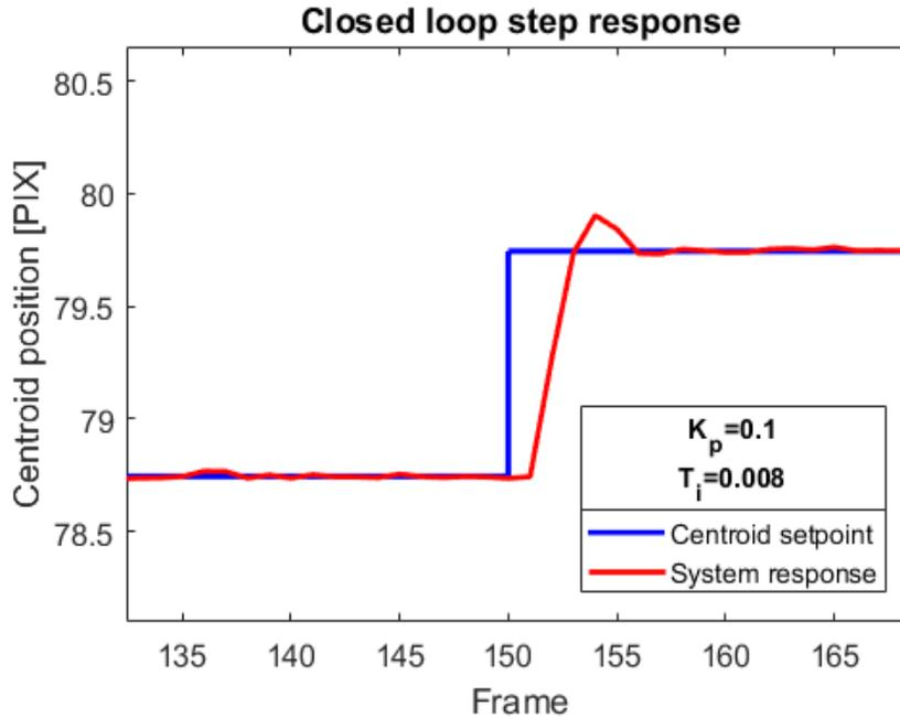
**Figure 34.** Closed loop step response with PI controller (framerate = 30 fps)
