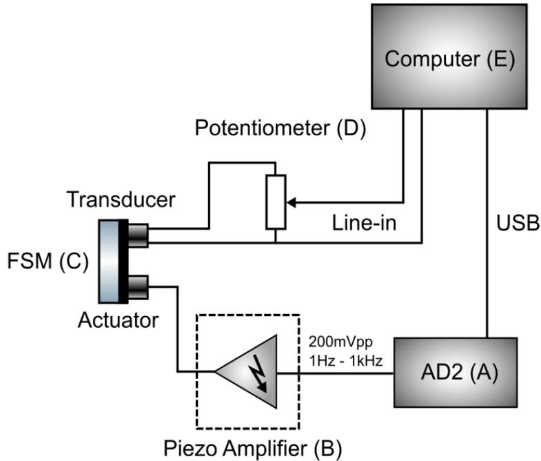
**Figure 29.** Setup for the determination of the steering mirror frequency response
