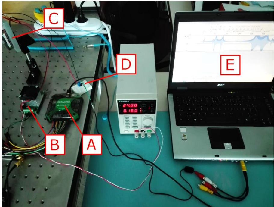
**Figure 30.** Photograph of the frequency response measurement setup
