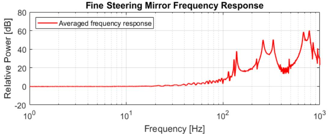
**Figure 31.** Steering mirror frequency response
