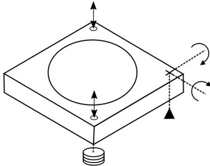
**Figure 17.** Steering mirror tip-tilt configuration
