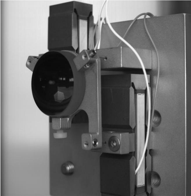
**Figure 19.** Front facing view of the steering mirror
