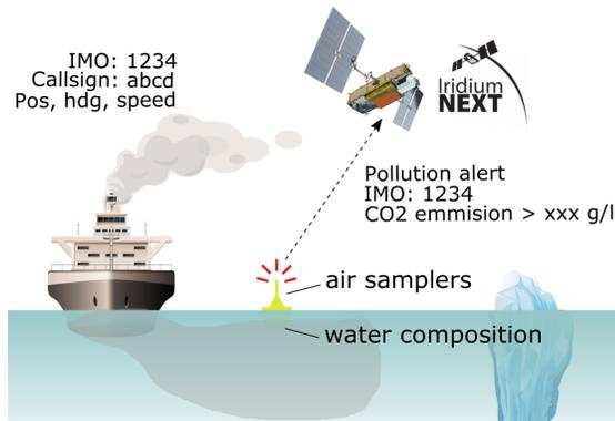
**Fig. 2:** Working principle of pollution detection by smart buoys along shipping lanes and AIS ship information relay via Iridium
